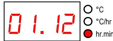
If a delayed start has been set then pressing the START/STOP key causes a time delay to start. The time remaining is shown on the display—this counts down once per minute. The Delay lamp on the mimic panel will light. The centre decimal point will flash once per second.
