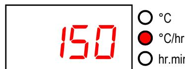
**►** then displays the ramp rate in the range 1 to 999°C/hr or *FULL* or *End*. This can be altered with the **↑** & **↓** keys. The Heating or Cooling lamp on the mimic display will flash.
