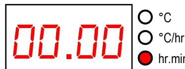
The next push of the **►** key displays the start delay time in the range 00.00 to 99.59 (99 hours 59 mins). This can be altered with the **↑** & **↓** keys. The Delay lamp on the mimic display will flash.
