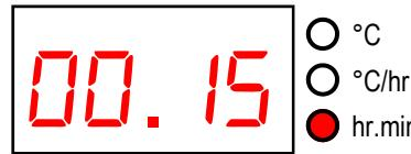
The next push of the **►** key displays the soak time in the range 00.00 to 99.59 (99 hours 59 mins). This can be altered with the **↑** & **↓** keys. The Soaking lamp on the mimic display will flash.
