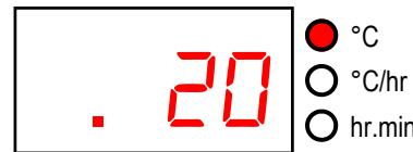
If the left-hand decimal point is on then the keyboard is locked & the ST315 will not respond to the START/STOP key. Press the **↑** & **↓** keys together & hold down for 5 seconds to unlock.
