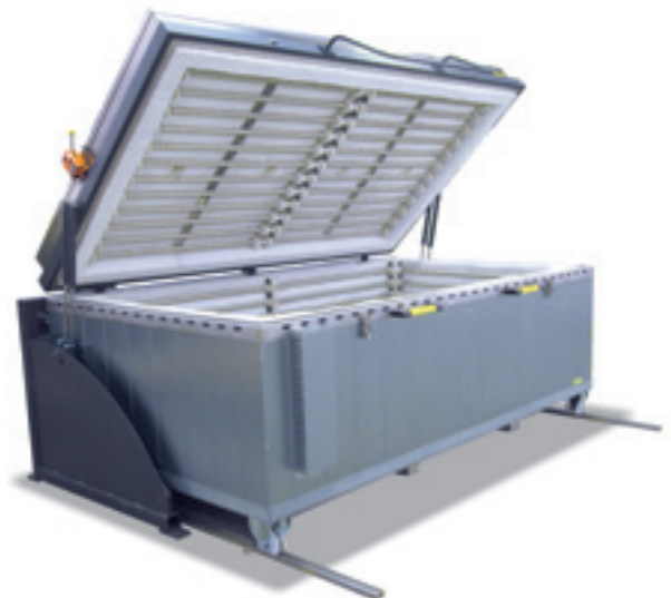
Top hat furnace with rail-mounted, movable trough
