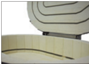
Kiln interior with circular lower side heating
