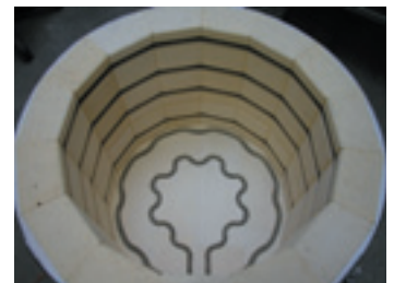
Bottom heating for Top 140 and Top 190
