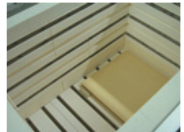
Firing chamber with heating from 5 sides
